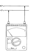
$^{\circ}$  Read off the measured value: in the case of DC voltage, on the two upper scales 0 ... 5 or 0 ... 15 V, A  $_{=}$  , in that of AC voltage, on the scales beneath 0 ... 5 or 0 ... 15 V, A  $\sim$  .
